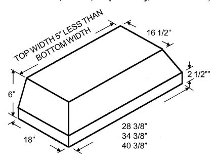
The VP521 transition is available for top vent applications at an additional charge.
