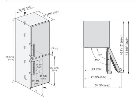
\* Dimensions without wall spacers installed. The appliance depth is increased by 9/16" (15 mm) with the wall spacers supplied installed.
