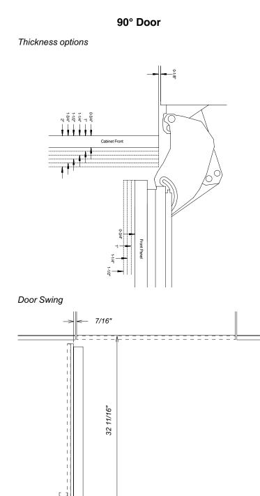
**NOTE**: Additional space needed depending on thickness of front panels and handle used
