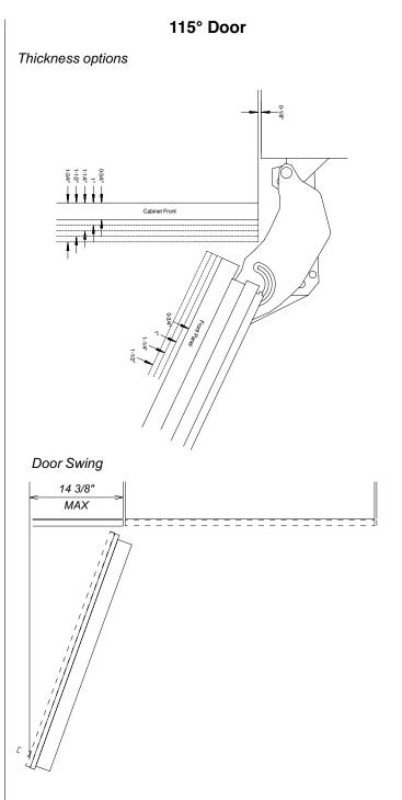
**NOTE**: Additional space needed depending on thickness of front panels and handle used
