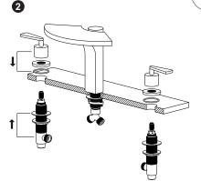
Install valve 8 into specified drill hole underneath the counter top. Place o-ring 4 into the base plate 3. Screw base plate 3 and the valve cover 2 into valve 8. Adjust the height and position of valve 8, then screw fixing ring 7 to tighten valve 8 underneath counter top securely. Install handle 1 to handle connector 5 of valve 8. Tighten set screw 20 with alley key and then place decorative cap 19 on handle 1.
