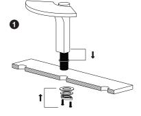
Fit O-ring 10 into the bottom groove of faucet body 9. Insert faucet body 9 into specified drill hole (1 1/4"- 1 ½") on the counter top. Install washer 11 and brass washer 12 to the threaded tail pipe of the faucet body 9 from underneath the counter top and then screw the fixing ring 13. Fix faucet body 9 correctly and install the three way connector 16 by screwing onto the threaded tail pipe of the faucet body 9.
