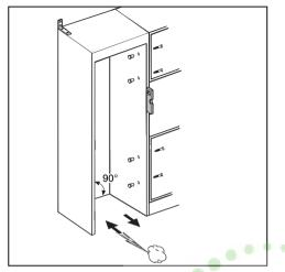
The housing unit must be carefully aligned using a spirit level before installing the appliance. The unit corners must be at right angles, as otherwise the furniture door will not Appliance Authority align correctly with the 4 corners of the appliance.
