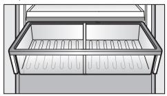
On the hinged side of the door is a safety lock, which must be turned to a horizontal position before the drawer can be removed.
