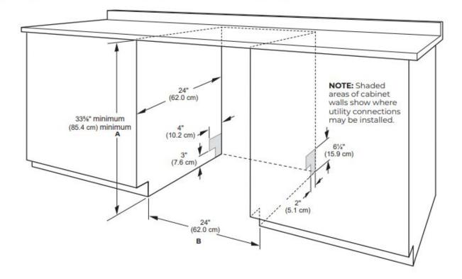
A. Measured from the lowest point on the underside of the countertop. May be reduced to 33%" minimum (85.4 cm) minimum by removing the feet and perforated area of insulation (blanket) on dishwasher.
