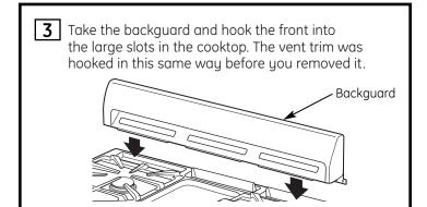
Rotate the backguard into place. Make sure that the center vent is clear upon installation.
