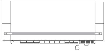
10. Install the over-the-range microwave with side panels into the 36" opening.
