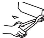
\* **IMPORTANT:** If a rectangular-to-round transition adaptor is used, the bottom corners of the damper will have to be cut to fit, using the tin snips, in order to allow free movement of the damper.
