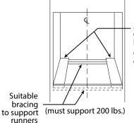
2 x 4 or equivalent runners level with bottom of cutout and flush with sides of cutout or solid bottom floor.
