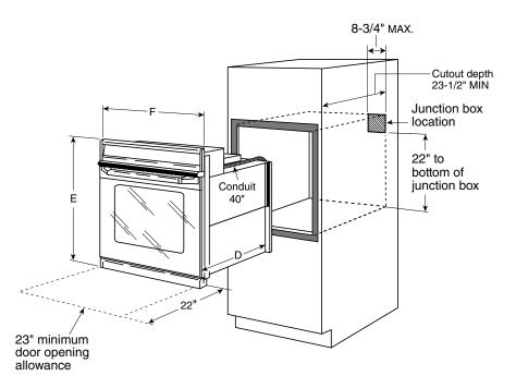
2 x 4 or equivalent runners level with bottom of cutout and flush with sides of cutout or solid bottom floor.
