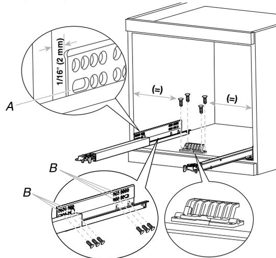
A. Front of mounting bracket 1/16" (2 mm) from outside of cabinet frame
