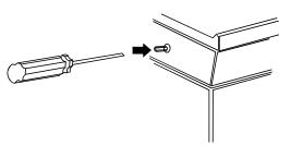
Center adjustment screw for all burners.
