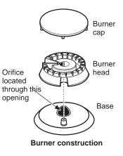
B. Using a 7 mm or 9/32" nut driver, remove the top burner orifices. These may be accessed through the burner opening in the base.
