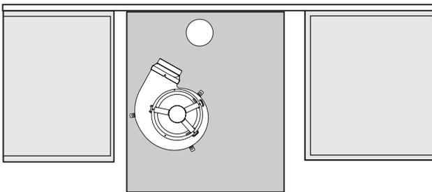
7. Connect the house vent system to the blower outlet adapter using a vent clamp; then wrap connection with aluminum tape.
