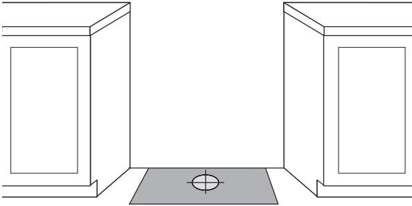
2. Draw and cut the vent hole in the floor.
