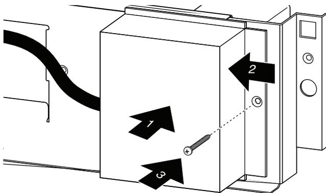
10. Replace the access panel by aligning the studs with the keyhole slots on the range. Press the access panel forward into the slots and push downward to engage the studs.
