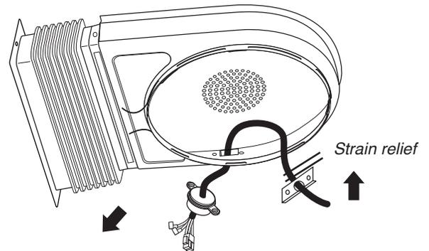
3. Feed blower motor wire through opening and place the strain relief bracket to the inside of the blower cover. Install and tighten the two (2) provided #8–18 x 3/8" screws to secure the strain relief bracket.
