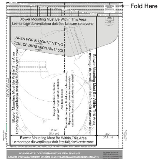
**NOTE:** The template has lines every 1/4" (6.4 mm) from the back edge. If the distance measured in the previous step is 1 1/4" (32 mm), fold the template on the line labeled 1 1/4" (32 mm). If there is no countertop filler depth, fold the template at zero depth.
