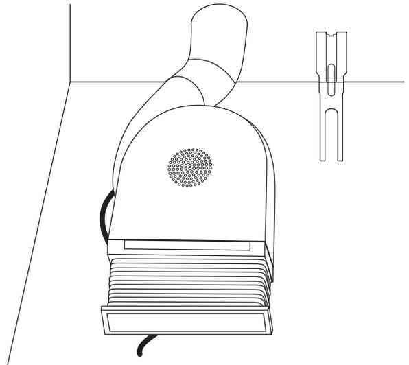
8. Move blower motor wire to the front of the installation.
