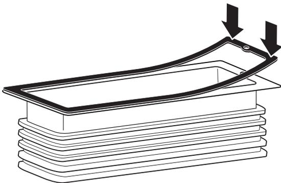
6. Apply blower motor cover to the blower. Slightly spread the cover retainer spring to allow the cover to drop into position on the blower motor.
