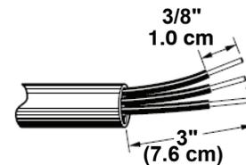
2. Allow enough slack in the wire to easily attach the wiring terminal block.
