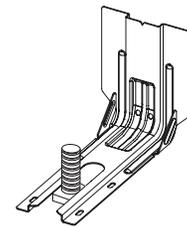
14. Rotate blower motor cover so the bellows are in their final position. Ensure the rear of the bellow flange is engaged in the retaining bracket.
