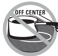
Always place the pan in the center of the surface unit you are cooking on.
