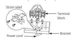
For 3/4" conduit installations only, purchase a squeeze connector matching the diameter of your conduit and assemble it in the hole. Insert the conduit through the squeeze connector and tighten. Allow enough slack to easily attach the wires to the terminal block. NOTE: Do not install the conduit without a squeeze connector. The squeeze connector MUST be installed before reinstalling the rear range wiring cover
