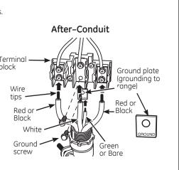
NOTE: Aluminum building wire may be used but it must be rated for the correct amperage and voltage
