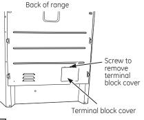
For power cord installations only **B** For power cord and 1" conduit only, remove the (see the next step if using conduit) assemble the strain relief in the hole. Insert knockout ring (1¾") located on bracket directly the power cord through the strain relief and tighten. Allow enough slack to easily attach the cord terminals to the terminal block. If tabs are present at the end of the winged strain relief, they can be removed for better fit.
