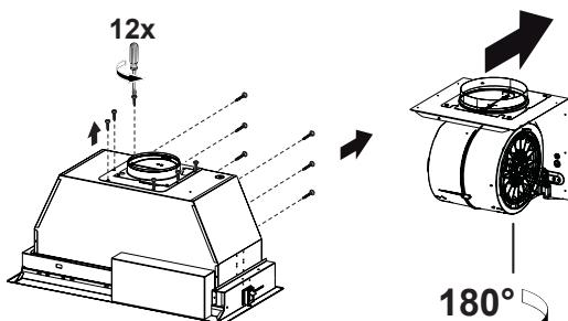
For a horizontal ducting installation the motor needs to be unsecured by first removing the 12 screws as shown.
