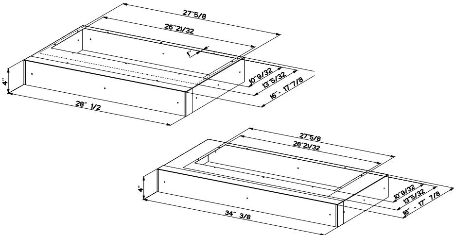
"Note: Standard Liners need to have the center perforation removed for installation"
