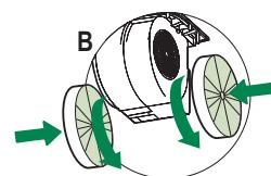
**Caution:** "When used in recirculation mode, to Reduce the Risk of Fire and Shock use only conversion kit Model FILTER 1 or FILTER1LL"
