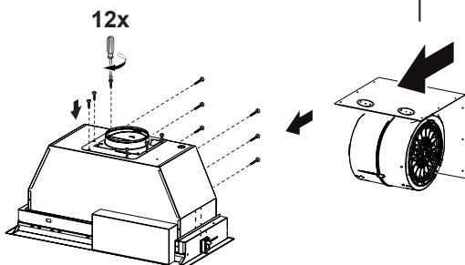
Once the blower is in place re-install the 12 screws to fasten the motor to the Insert Hood body.
