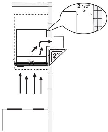
For horizontal(rear) ducting there must be a minimum of 2 1/2" of space open between the back of the Hood Insert and the wall.
