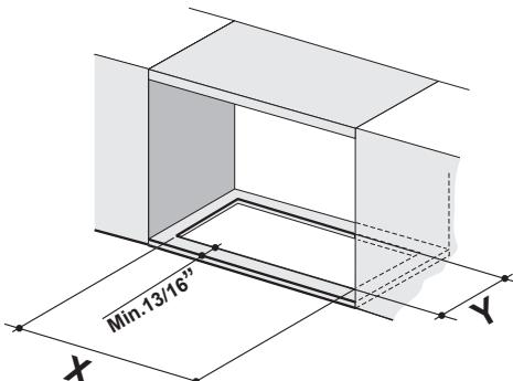
Cut out the opening in the underside of the cabinet as shown in Figure 1.
