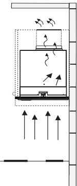
For Non-Ducted Recirculation venting route the ductwork to a location above the hood where the discharge is vented back into the room.
