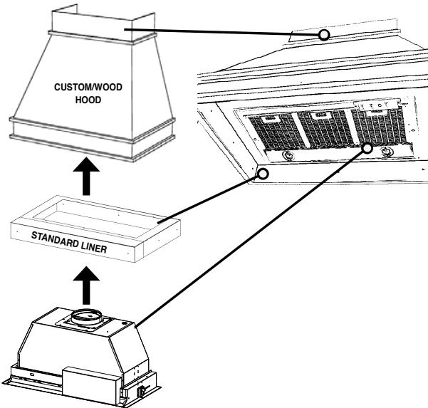
1. The custom/wood hood must have a sturdy base (3/4" plywood recommended) to accommodate the cut-out for the Inca HC. The base must be recessed to accommodate the height of the Liner (see **LINER DIMENSIONS** on Page 13). The Liner attaches to the bottom of the base using screws appropriate for the size and material of your custom/ wood hood. The Inca HC inserts into the cut-out in the Liner and base.
