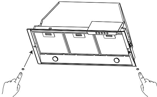
Insert the 2 Caps in the screws hole, as shown.
