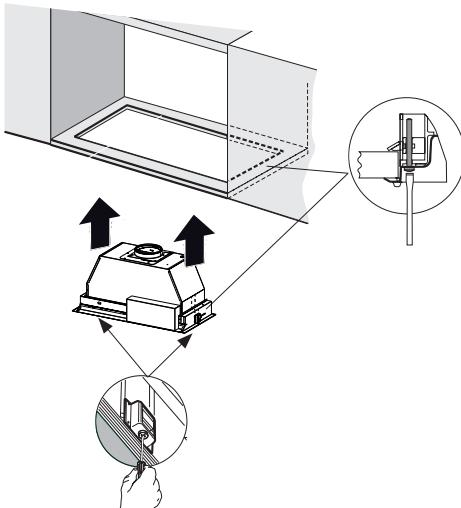
Install the Insert Hood through the cabinet cutout into the cabinet opening that has a minimum height of 16". Allow for ducting.
