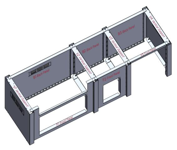
Using the provided screws, fasten each Support and Panel together in the corners of each section.
