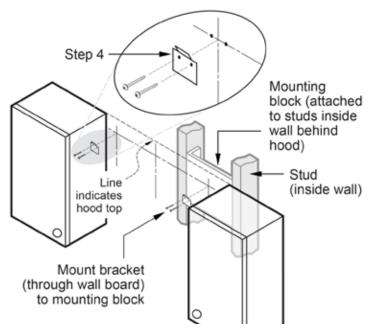
Attaching the Brackets to the Wall
