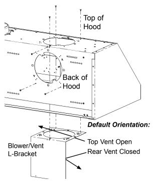
2. Turn and align the L-bracket so the hole is in back of the hood, allowing a rear-venting configuration.
