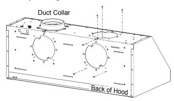
3. Remove the duct collar from the hood top. (Save the collar and screws.)
