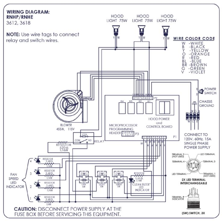
Wiring Diagram: 1-Blower, 3-Light Models
