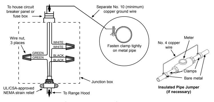
**Grounding by External Cold-Water Pipe**
