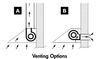
Typically, the blower vents through hood top (A, above); however, the blower can be rotated to vent through the hood **rear** (B). When planning ductwork, always find the shortest, most direct route to the outside.
