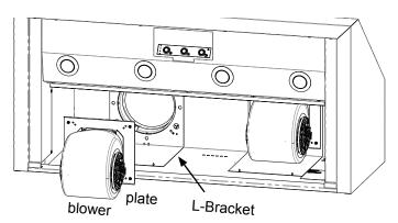
2. Find the end of the cable assembly plugged into the bottom left of the blower, then squeeze and unplug the connector. (To avoid damaging the cable assembly contacts and wires, *always* pull by the connector.)
