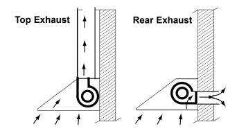
The blowers (fans) can be rotated so air vents out the back of the hood.
