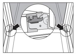
The oven door is connected to the hinges by retainers.
