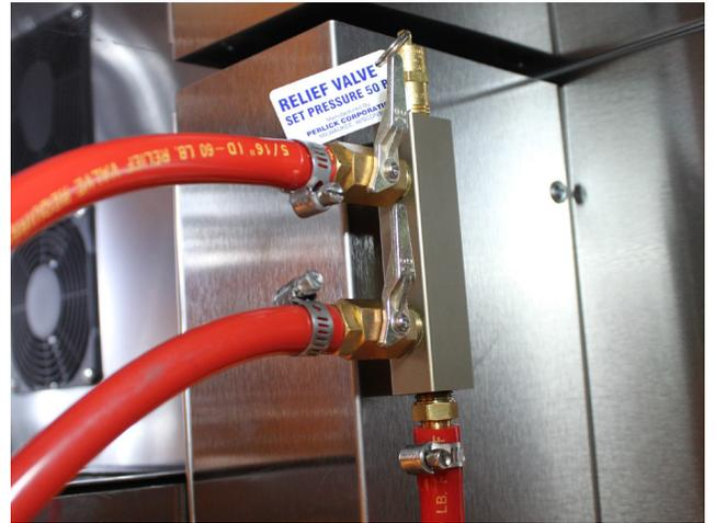
5. On a single beer system, locate the red CO2 hose. Slide one end onto the barbed fitting of the regulator assembly and clamp. On systems with two or three beers, locate the CO2 line that comes off the backside of the manifold assembly. Slide the hose onto the barbed fitting of the regulator assembly and clamp. For detailed information on connecting the regulator to the CO2 cylinder, see page 8.
