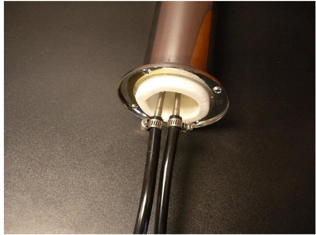
2. Insert the beer line(s) through the hole in the counter top. Position the head in place and apply silicone around the base of the dispensing head. Fasten using the 4 chrome screws included with the dispensing head. Wipe off excess silicone to complete the seal.
