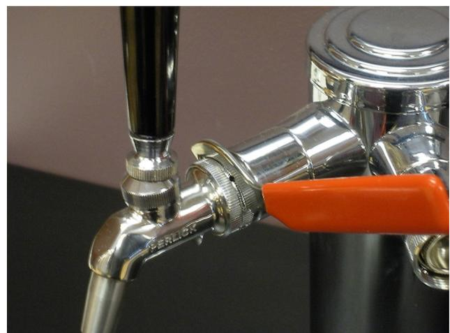
10. Before tapping, make sure the beer faucet is closed. To tap a keg, insert the coupler into the fitting on top of the barrel. Turn the coupler clockwise until it stops (about an 1/8 turn), then push down on the top of the coupler and again turn clockwise until it stops. Your barrel is now open. Open the CO2 valve on the regulator as well as the valve on the manifold if used. Using soap and water solution, check all CO2 connections for leaks indicated by bubbles. Tighten as needed.
