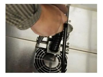
If installing a two faucet system, a CO2 manifold will need to be installed. Locate the red CO2 lines, CO2 manifold and a #10 x 1/2" sheet metal screw. Slide one end of each hose onto the barbed fittings on the manifold and clamp. On the left rear side wall of the beer compartment there is a double row of screws which run vertically. Remove one of the two top screws and discard. Insert the sheet metal screw through the manifold and into the hole vacated previously.
