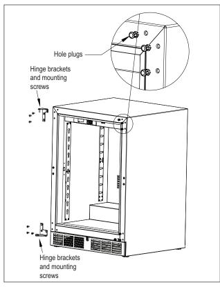
Figure 8. Hinge Removal
