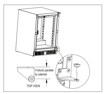
Figure 15. Installing V-Block
