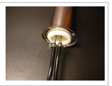
2. Insert the beer line(s) through the hole in the counter top. Position the head in place and apply silicone around the base of the dispensing head. Fasten using the 4 chrome screws included with the dispensing head. Wipe off excess silicone to complete the seal.
