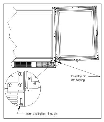
Figure 16. Installing Door
