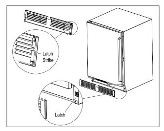
Figure 5. Toe Plate Installation
