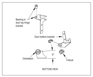
Figure 13. Bearing and V-Block
