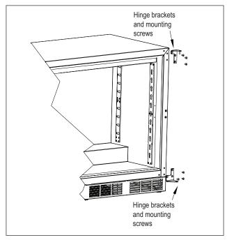
Figure 9. Hinge Installation
