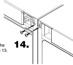
**14.** Attach the connecting plate supplied with the SBS Kit and fasten with the screws of step 13.
