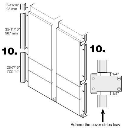
Adhere the cover strips leaving a gap of 1/4" to each securing plate to prevent interference when installing the covers.
