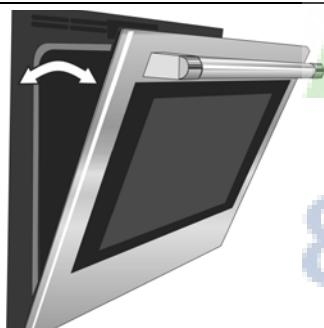
4. Holding the door firmly on both sides and using both hands, close the door gently until it stops against the levers, about 30° from the closed position.
