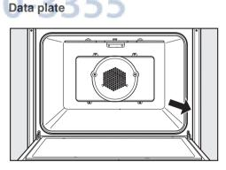
The silver data plate is located along the front side of the oven with the door open.
