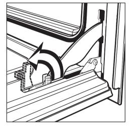
Slowly shut the door until the protruding clamps stop the movement. Pull the door upward. See illustration.
