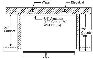
\*The rough-in dimension of 70-3/4" is minimum and is measured from the finished floor to top of opening (or the underside of the overhead cabinets). For Models with Trim Kit: If frameless style cabinets are planned for above the refrigerator, you may need to consider adding a maximum of 1/4" (71") to height of opening to allow additional clearance between cabinet doors and top of refrigerator trim when cabinet doors are in open position.
