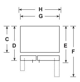
$\ensuremath{^\dagger} \xspace$  Water hook-up fits in back air clearance when calculating installation depth.
