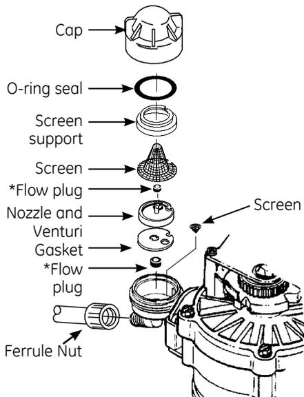
**IMPORTANT:** Be sure small holes in the gasket are centered directly over the small holes in the nozzle and venturi housing.
