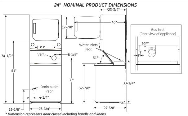
NOTE: With feet set at mid position, feet can be adjusted ±.375".
