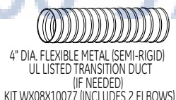
4" DIA. METAL DUCT (RECOMMENDED)
