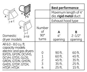
For every extra  $90^\circ$  elbow, reduce the allowable vent system length by  $10\,\mathrm{ft}$ .
