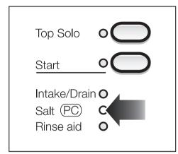
After the reservoir has been filled, the water softener is automatically reactivated the next time the dishwasher is started. The "Salt" indicator will be lit during this process.
