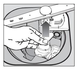
Pull out the non-return valve and rinse well under running water.
