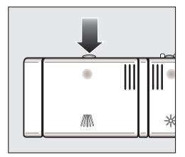
■ To open, press the latch on the detergent dispenser. The flap will spring open.
