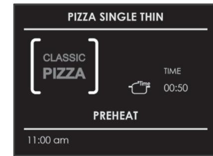
NOTE After the first pizza, you can immediately continue baking other pizzas without having to preheat. If, on request is selected, the recipe is repeated, while if OFF is pressed the recipe terminates.
