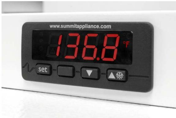
When the cabinet reaches 140°F, the heating element will turn off (the red light goes out), then turns on again when the cabinet temperature drops to 135°F. This condition will continue until the equipment is turned off intentionally or:
