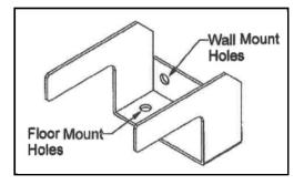
The bracket will be positioned at the back of the appliance, 1<sup>1</sup>/<sub>4</sub>" from the left edge (as you face the front). Holes should be drilled at 1-13/16" and 3-9/16" from the left edge of the unit. Drill into a suitable foundation, either wood studs or joists. <u>The bracket must not be screwed into sheetrock</u>.
