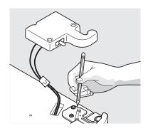
2 Remove the two screws from the top hinge. Lift the door off of the bottom hinge and set it aside.
