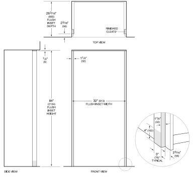
\*3" (76) typical depth. Shaded areas will be visible and should be finished to match cabinetry. NOTE: Shaded line represents profile of unit with <sup>3</sup>/4" (19) panel.
