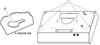
**2.**Use 1/8'' (3 mm) drill bit and drill 4 pilot holes as shown. NOTE: Make the drill holes on the thin area of the slot.
