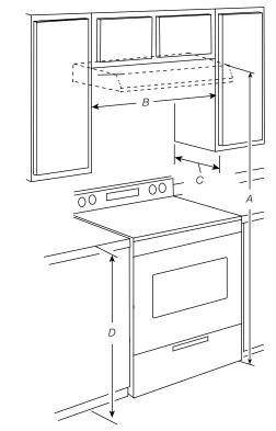
A. 66'' (167 cm) suggested min. - top of range hood to floor. B. 30'' (76.2 cm) min. cabinet opening width for 30'' (76.2 cm) models and 36'' (91.4 cm) min. cabinet width for 36'' (91.4 cm) models.
