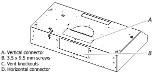
**5.** Install the  $3\frac{1}{4}$ " x 10" (8.3 x 25.4 cm) vent connector. Attach to range hood with the .35 x .95 cm screws that you previously removed (step 1) and remove tape from damper flap.
