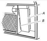
**3.**Remove the power supply knockout from the top or rear of the vent hood (depending on the incoming location of your home power supply cable) and install a UL listed or CSA approved 1/2" strain relief.
