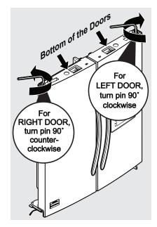
Once the door pins are reset, follow the steps "To reinstall the refrigerator doors".
