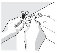
3 Detach the water tube from the connector located behind the refrigerator, the connector releases when you press inward on the connector's outer sleeve. Pull the water tube out toward the front of the unit.
