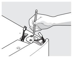
2 Disconnect the harness by grasping both sides of the connector firmly, depress the latch and pull apart.
