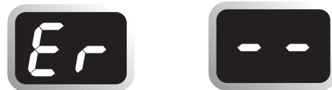
Figure 7: Er indicator message (L) and ESEC lockout feature (R)
