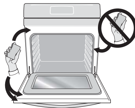
Figure 39: Clean around the oven door gasket
