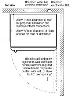
\* When installing refrigerator adjacent to wall, cabinet or other appliance that extends beyond front edge of unit, 20" minimum clearance recommended to allow for optimum 140° door swing, providing complete crisper access and removal. (Absolute 3" minimum clearance will ONLY allow for 90° door swing which will provide limited crisper access with restricted removal.)
