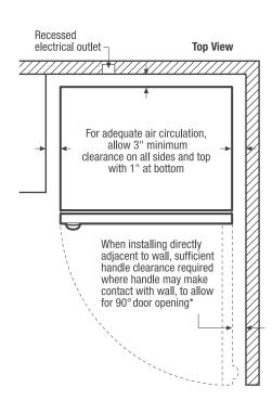
\* When installing refrigerator adjacent to wall, cabinet or other appliance that extends beyond front edge of unit, 20" minimum clearance recommended to allow for optimum 140° door swing, providing complete basket access and removal. (Absolute 3" minimum clearance will ONLY allow for 90° door swing which will provide limited basket access with restricted removal.)
