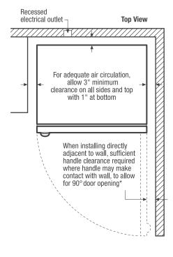
\* When installing refrigerator adjacent to wall, cabinet or other appliance that extends beyond front edge of unit, 20" minimum clearance recommended to allow for optimum 140° door swing, providing complete basket access and removal. (Absolute 3" minimum clearance will ONLY allow for 90° door swing which will provide imited backet access with restricted removal. limited basket access with restricted removal.)
