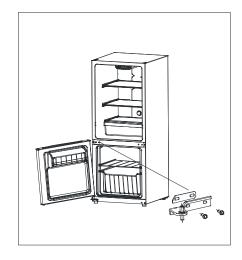
7) Place the refrigerator door on the middle hinge. Be sure the door is aligned horizontally and vertically, and that the gasket seals on all sides before attaching the top hinge. Attach the top hinge and replace the hinge cover.
