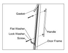
3. Replace the door gasket to its original position.
