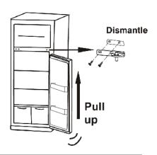
Remove the screws from the middle hinge. Lift the refrigerator door up and away from the appliance.
