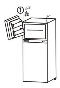
Place the freezer door on the middle hinge. Ensure that the door is aligned horizontally and vertically, and that the gasket seals on all sides before attaching the top hinge. Attach the top hinge and replace the hinge cover.
