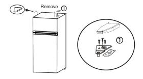
Remove the hinge cover. Unscrew and remove the top hinge.
