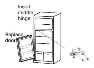
Remove right pin assemblies from the bottom of the freezer and refrigerator doors. On the opposite side, attach the replacement pin assemblies (located in the plastic bag with the Use and Care Manual) with a screwdriver.
