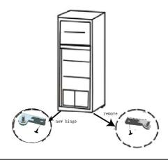
Remove right bottom hinge and reserve the screws. Remove screw covers at left corner and put them into the screw holes at right corner. Install left hinge by using those reserved screws.
